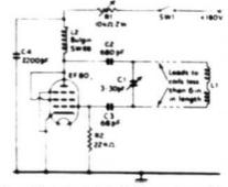
sides of the neck, immediately behind the main coils, and may have to be within the focus yoke. The length of the leads to the oscillator should not be more than 6". The oscillator frequency is tunable around 12.5Mos, condenser Cl being adjustable to avoid IP beats and spurious patterning.
